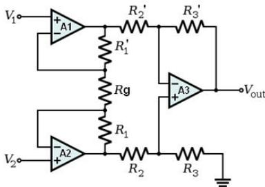
Fig 2. Voltage-Mode Instrumentation Amplifier
