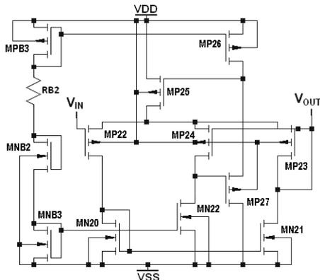
Fig 8. Analog Buffer
