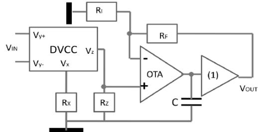
Fig 3. Designed Instrumentation Amplifier
