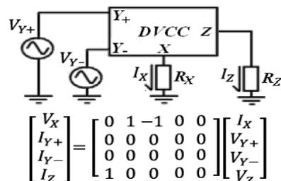
Fig 4. DVCC Functional Block and Operational Matrix
