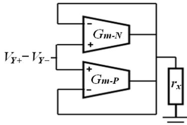
Fig 6. Complementary DVCC Block Diagram [8]
