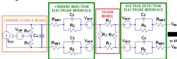
Fig 11. BI Front-End Interface Circuit
