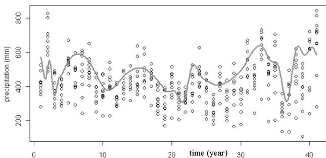
Fig. 7. The model for the precipitation variability in Dobrudja region, obtained by wavelets method (hard threshold) using ten series
