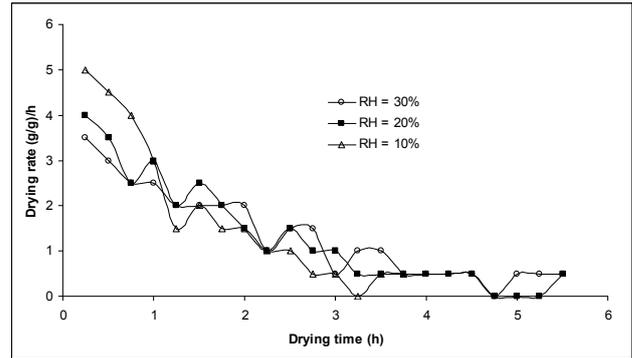
Fig. 5. Drying rate curves: dry basis moisture content versus drying time at 55 °C and air velocity of 1 m/s
