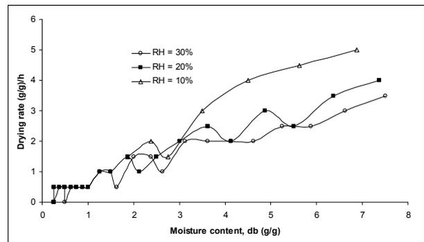
Fig. 6. Drying characteristic curves: a dry basis moisture content versus drying time at 55°C and air velocity of 1 m/s
