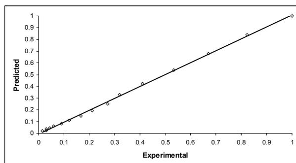
Fig. 10. Comparison of experimental MR with predicted MR from Page's model at 10% RH
