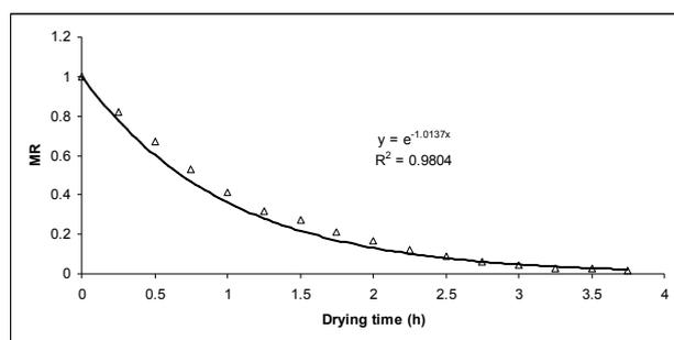
Fig. 7. Plot of MR versus drying time (Newton's model) at 10% RH
