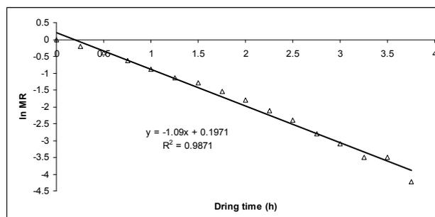
Fig. 9. Plot of  $\ln MR$  versus drying time (Henderson and Pabis model) at 10% RH
