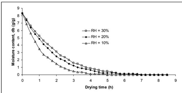
Fig. 4. Drying curve: dry basis moisture content versus drying time at 55°C and air velocity of 1 m/s
