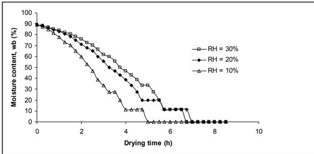
Fig.3. Moisture content variation with drying time at 55°C and air velocity of 1 m/s
