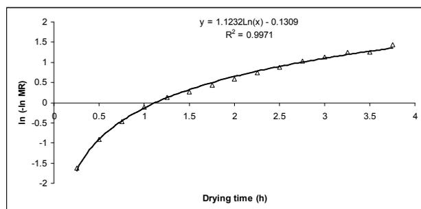
Fig. 8. Plot of  $\ln(-\ln MR)$  versus drying time (Page's model) at 10% RH
