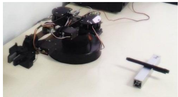
Fig. 2. Anthropomorphic Robot of 5 GDL
