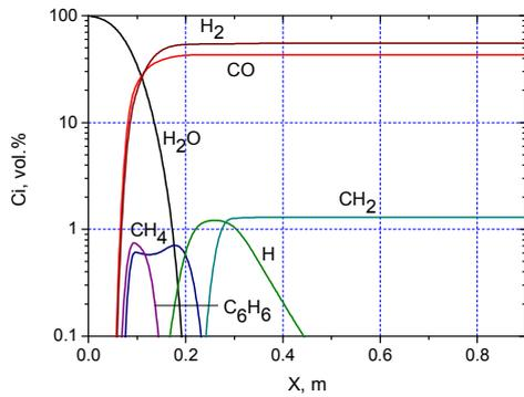
Fig. 2. Distribution of gas composition along the gasifier at EC gasification
