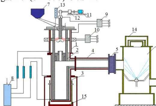
Fig. 1. Laboratory-scale plant for coals plasma gasification: 1 – plasma reactor; 2 – orifice, synthesis gas and slag separator chamber; 3 – slag catcher; 4 – synthesis gas cooling chamber; 5 – orifice; 6 – hydration chamber; 7 – dust feeder; 8 – cooling water system; 9, 10 – power supply system; 11, 12 – rod electrode moving system; 13 – steam generator; 14 – safety valve; 15 – slag catcher lifter
