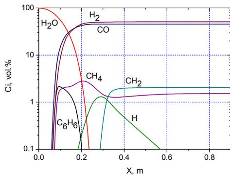
Fig. 3. Distribution of gas composition along the gasifier at SC gasification
