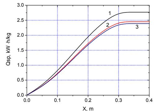
Fig. 6. Specific power consumption distribution along the gasifier: 1 – EC, 2 – SC, 3 – MC
