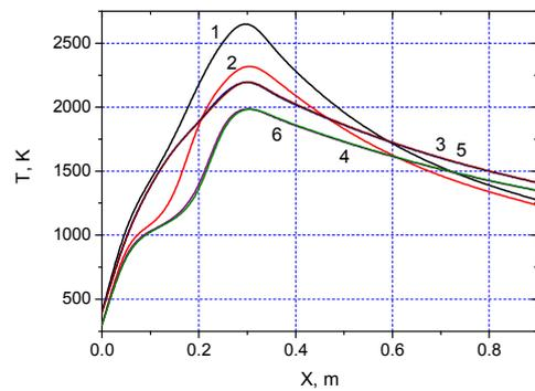
Fig. 5. Gas (1, 3, 5) and coal particles (2, 4, 6) temperature distribution along the gasifier: 1, 2 – EC; 3, 4 – SC; 5, 6 – MC
