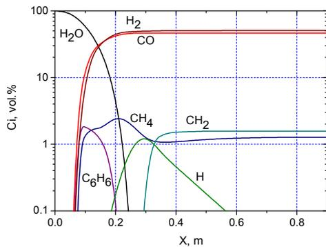
Fig. 4. Distribution of gas composition along the gasifier at MC gasification
