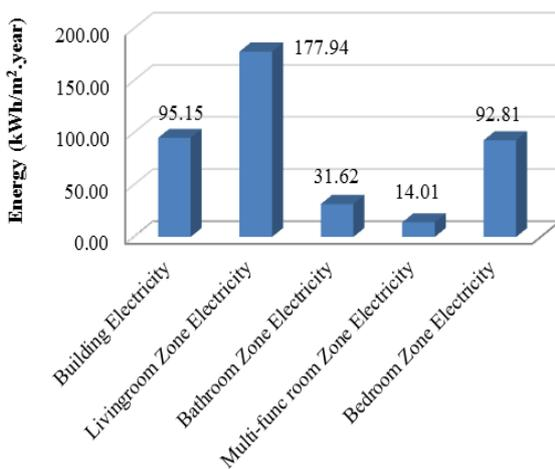
Fig.4. Electric energy consumption of the building and each zone
