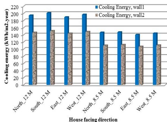
Fig. 5. Cooling energy of each house oriented with two wall materials; wall1: concrete block hollow, wall2: aerate concrete, and two operating modes of air conditioning unit
