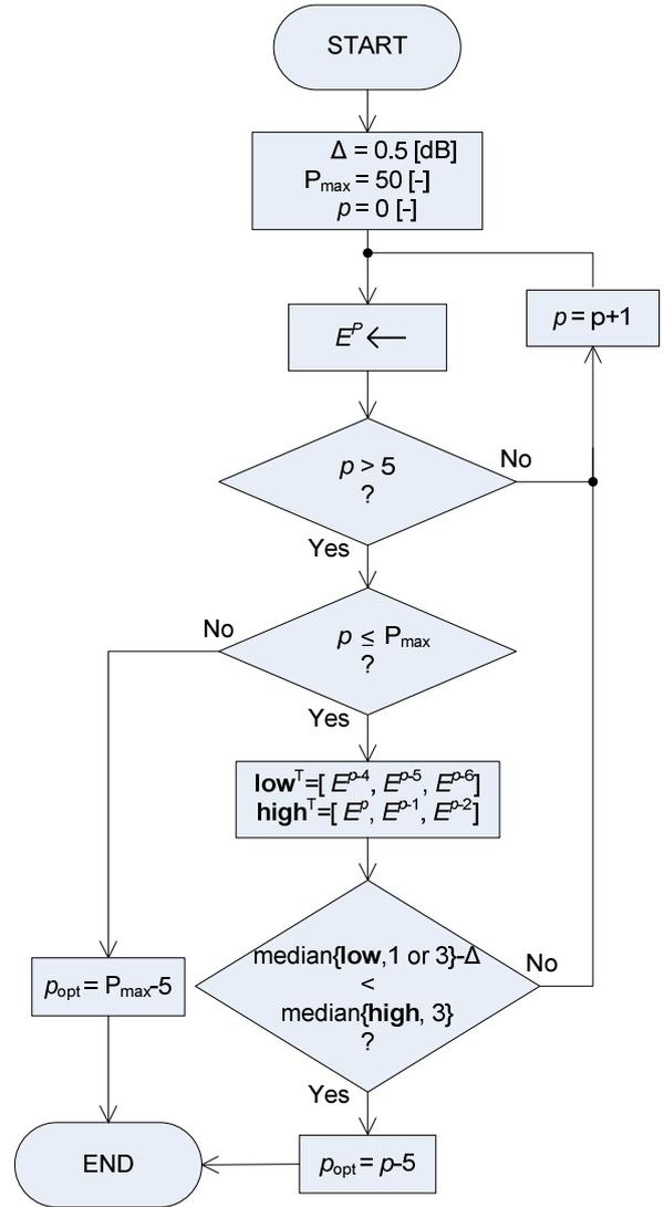
Fig. 5. Algorithm of optimal order  $p_{opt}(i)$  choosing method.
