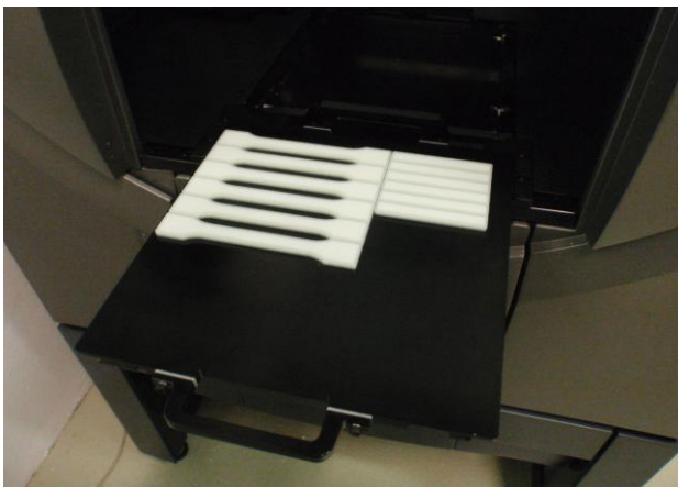
Fig. 4 Testing sample (for tensile tests) production (3D printing)
