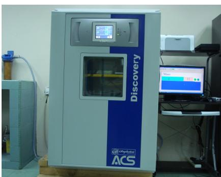
Fig. 1 photograph Constant Temperature and Humidity Chamber Test
