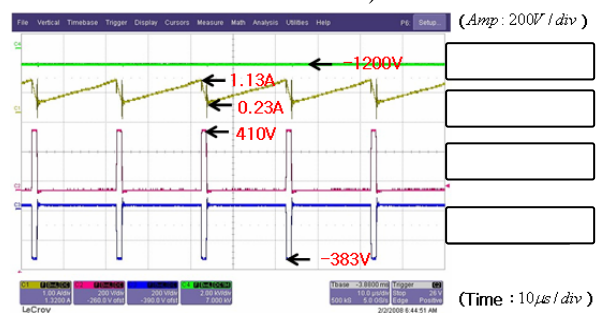
Fig. 9, Simulated Waveforms of the proposed circuit (3-Level circuit)
