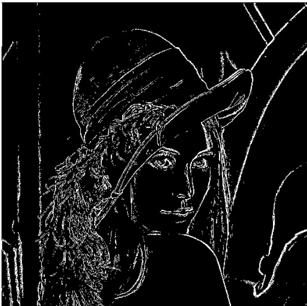
Figure 3: Top: Lena Image, Bottom: Detected edges using the Local Threshold and Boolean Function Based Edge Detection Algorithm
