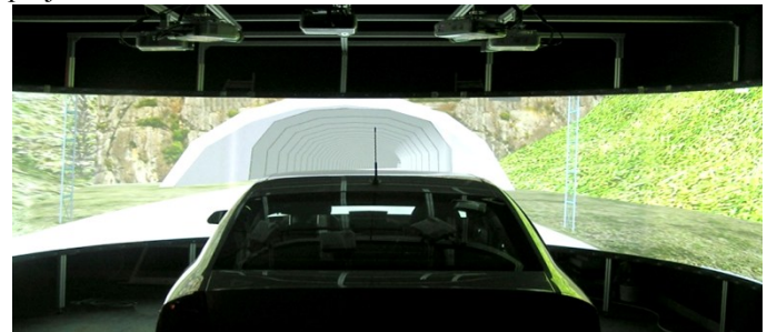
Fig. 1: Steady based full simulator with surrounding projection
