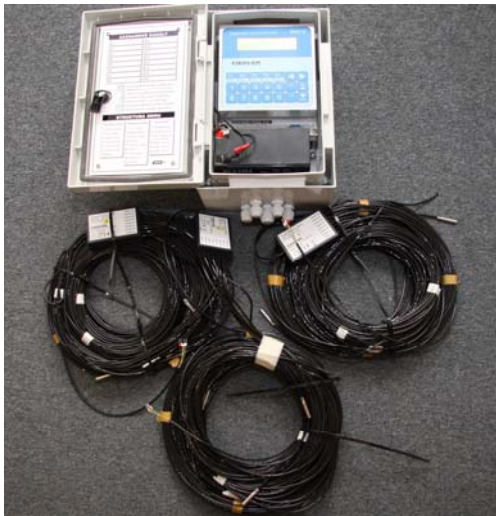
Fig. 2. Telemetric station with temperature sensors
