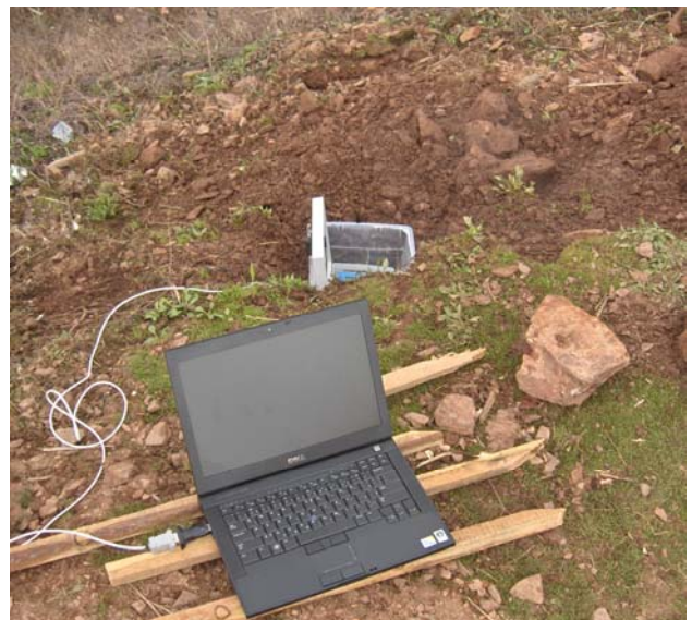
Fig. 8. A view of telemetric station configuration at the Ema mine dump
