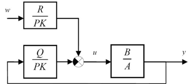
Fig. 2. 2DOF control loop
