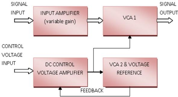
Fig.1, Circuit block diagram
