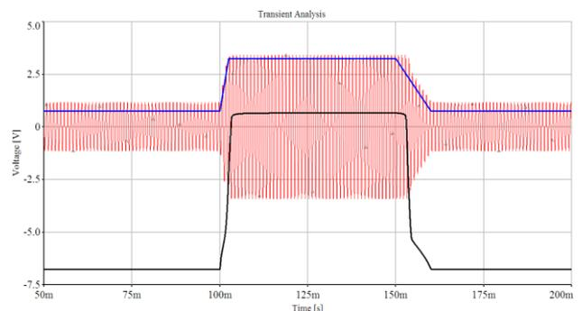
Fig. 9, VCA response to the input control voltage (fast sweep)
