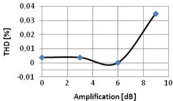
Fig. 10, Total harmonic distortion versus VCA amplification factor
