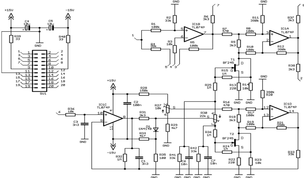
Fig. 4. Voltage controlled amplifier schematics (one of two channels)
