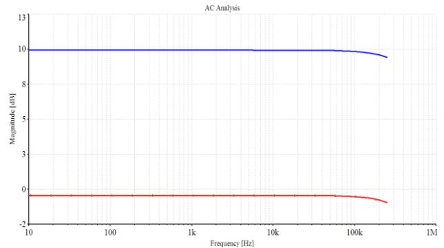
Fig. 7, The whole VCA frequency response at the pre-amplifier gain set to 0 dB and the VCA amplification factor set to 0 dB and + 10 dB
