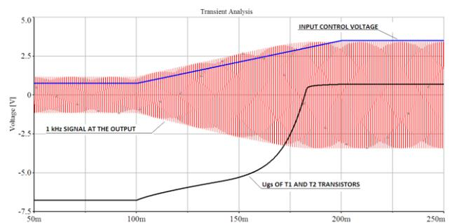
Fig. 8, VCA response to the input control voltage (slow sweep)
