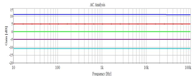
Fig. 5, Preamplifier frequency response at 5 different gain settings
