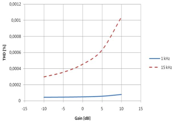
Fig. 6, Pre-amplifier distortion versus its gain setting
