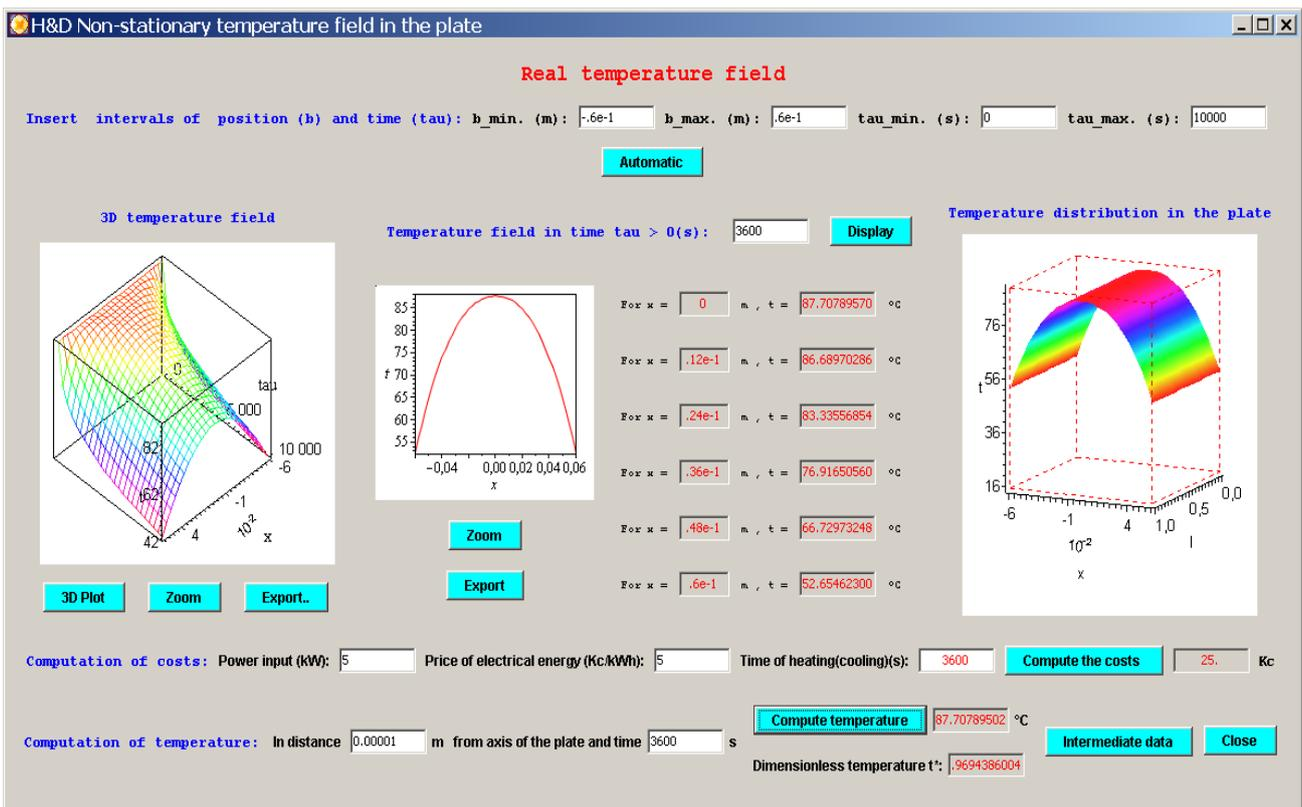
Fig. 4 The window for real temperature field computing
