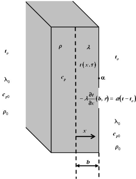
Fig. 1 Geometry sketch of the non-stationary symmetric heat conduction in a plane plate
