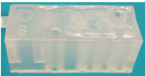
Fig. 11 Defects on part – sink marks (right)
