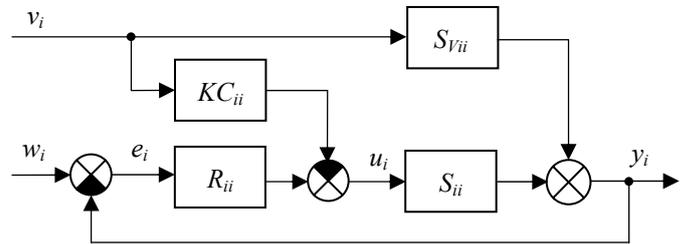
Fig.2 - Block diagram of SISO branched control loop with measuring of disturbance variable  $v_i$
