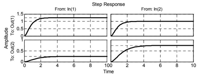
Fig.4 - Step response of transfer matrix of the controlled plant  $G_S(s)$
