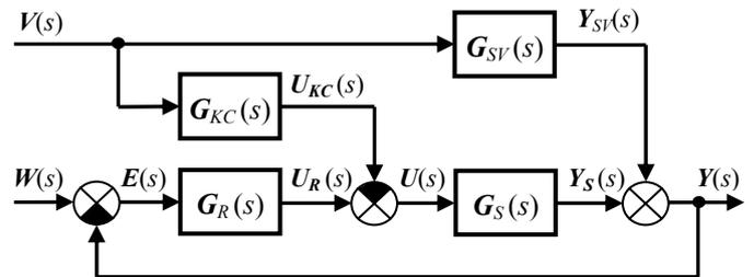
Fig.1 - MIMO branched control loop with measurement of disturbance
