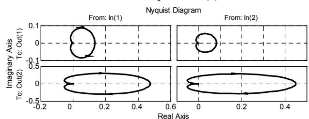
Fig. 7 - Nyquist diagram of transfer matrix of the disturbance variables  $G_{SV}(s)$
