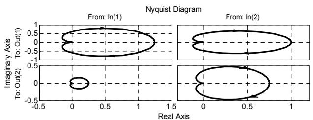
Fig. 6 - Nyquist diagram of transfer matrix of the controlled plant  $G_S(s)$
