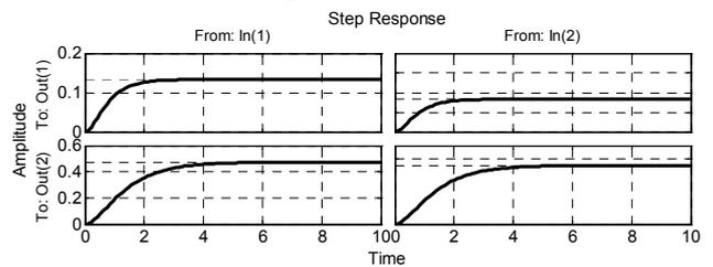
Fig.5 - Step response of transfer matrix of the disturbance variables  $G_{SV}(s)$
