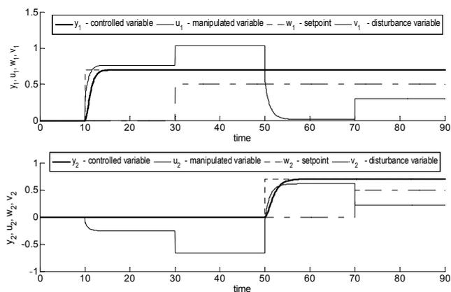
Fig.10 - Simulation course of control loop with utilization of pole placement method
