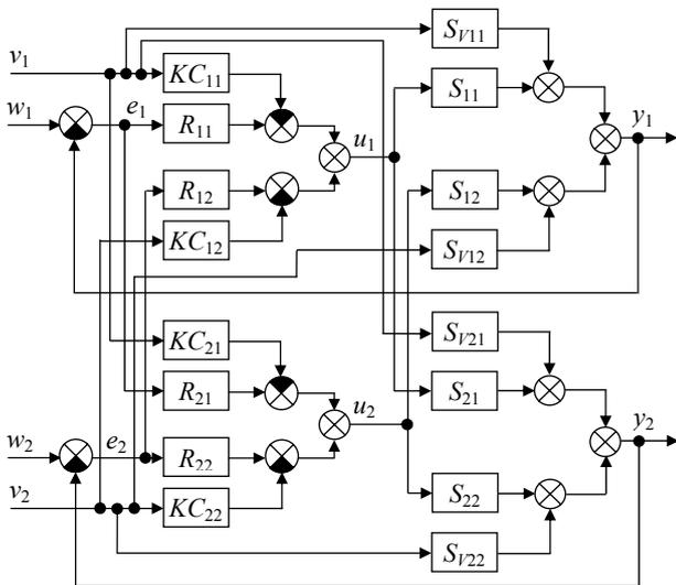
Fig.3 - Two-variable branched control loop with measurement of disturbance
