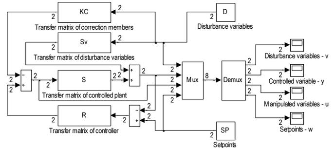
Fig.8 - Simulation scheme of two-variable control loop in the program MATLAB/SIMULINK
