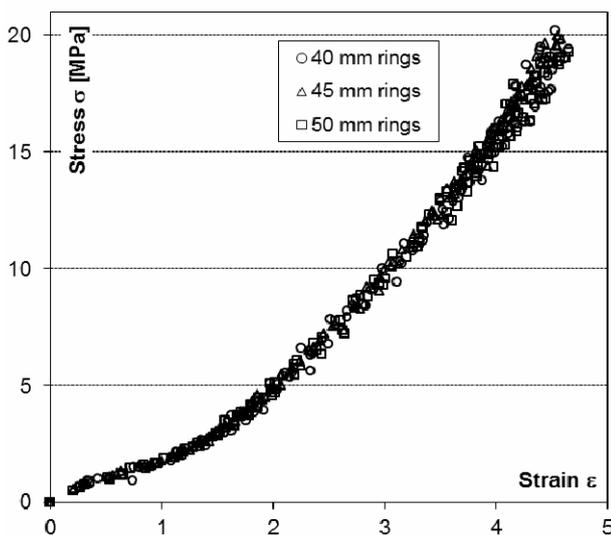
Fig. 4 Stress-strain diagrams for specimens with 1mm thicknesses clamped in all three rings
