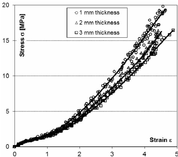
Fig. 3 Stress-strain diagrams for specimens of all three thicknesses clamped in the ring of 50 mm inner diameter
