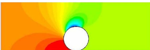
Fig. 6. Static pressure distribution at  $\tau = 120$  sec
