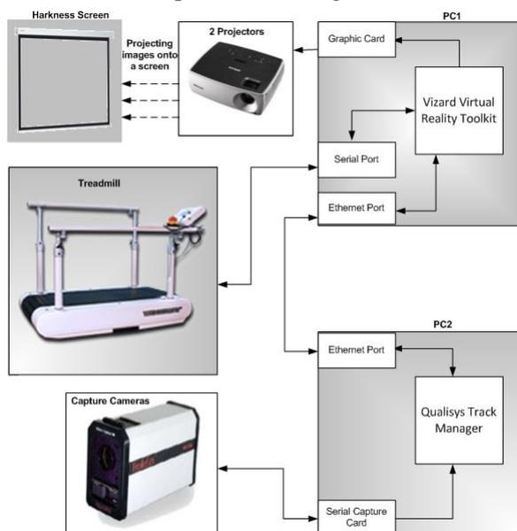
**Figure 3:** A block diagram of the SVRS
