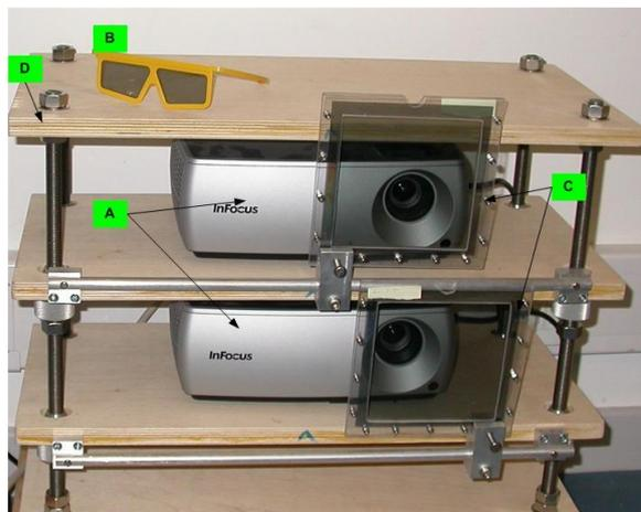
**Figure 2:** The main projection components of the SVRS. A: projectors; B: passive polarized glasses; C: circular passive polarising filters; and D: an in-house developed projector stand
