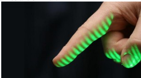
Fig 3. Flashscan's fingerprinting uses stripes of light to capture a 3D image with no touching
