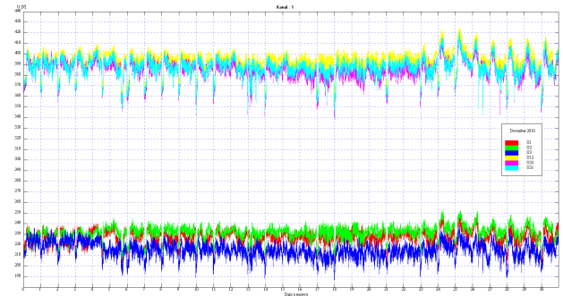
Figure 7. Phase and line voltages recorded on a pole of TS 10/0.4 kV "N. Tesla 2" LV feeder - December 2010.
