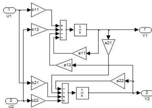
Fig.7 Schematic for modeling system by the third approach
