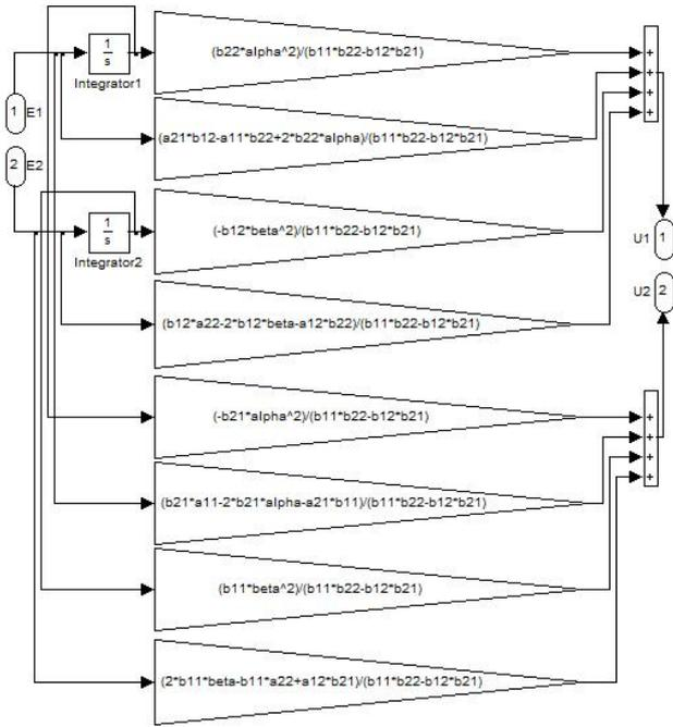
Fig.8 Schematic for modeling of the controller by the third approach
