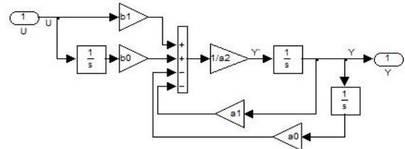
Fig.6 Subsystem block representing partial transfer function  $G_{11}$
