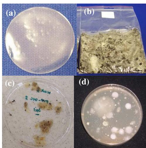
Fig.3: Biodegradability of PVP-CMC hydrogel film (a) hydrogel film before degradation, (b) compost bed where the film was buried for degradation, (c) hydrogel film after biodegradation (after 4 weeks degradation), (d) an image of microbes which are present in compost bed.
