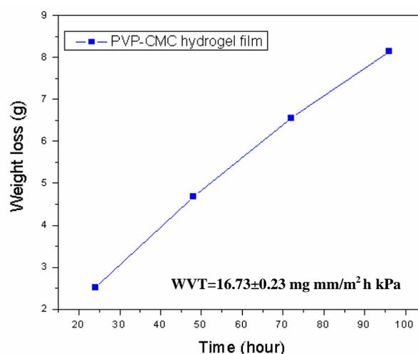
Fig. 2: Profile of water vapour transmission through PVP-CMC hydrogel film
