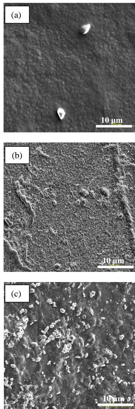
Fig. 4: SEM micrograph of PVP-CMC hydrogel film. (a) Initial and after (b) 2 weeks and (c) 4 weeks of bio-degradation.
