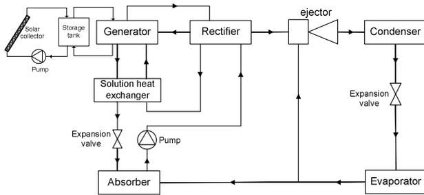
Fig. 1 Schematic of the experimental setup concept
