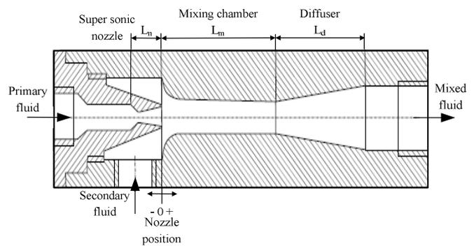
Fig. 3 The ejector used in the experimental setup
