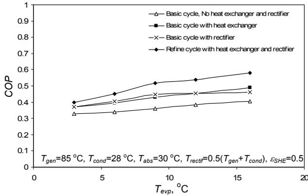
Fig. 5 Variation of *COP* with evaporator temperature (conventional system)
