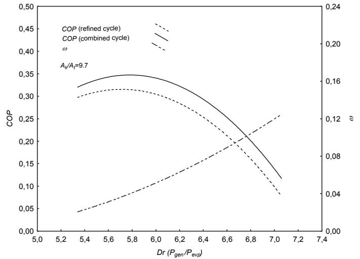
Fig. 7 Comparison of *COP* and *w* for both conventional and combined system
