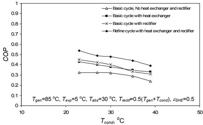
Fig. 6 Variation of *COP* with condenser temperature (conventional system)
