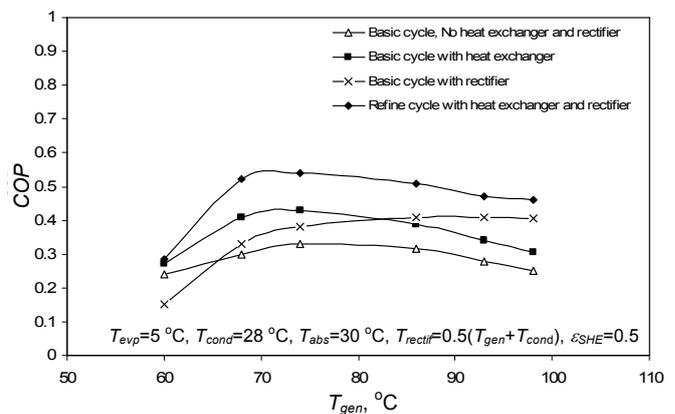
Fig. 4 Variation of *COP* with generator temperature (conventional system)
