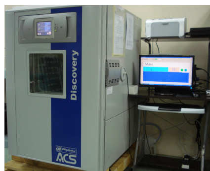
Fig. 1 Photograph Low Temperature and Humidity Chamber Test
