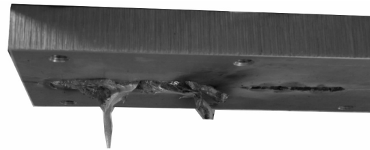
Fig. 5: Root side of a 20 mm thick welded aluminum alloy 5754 without (left) and with electromagnetic support system (right).
