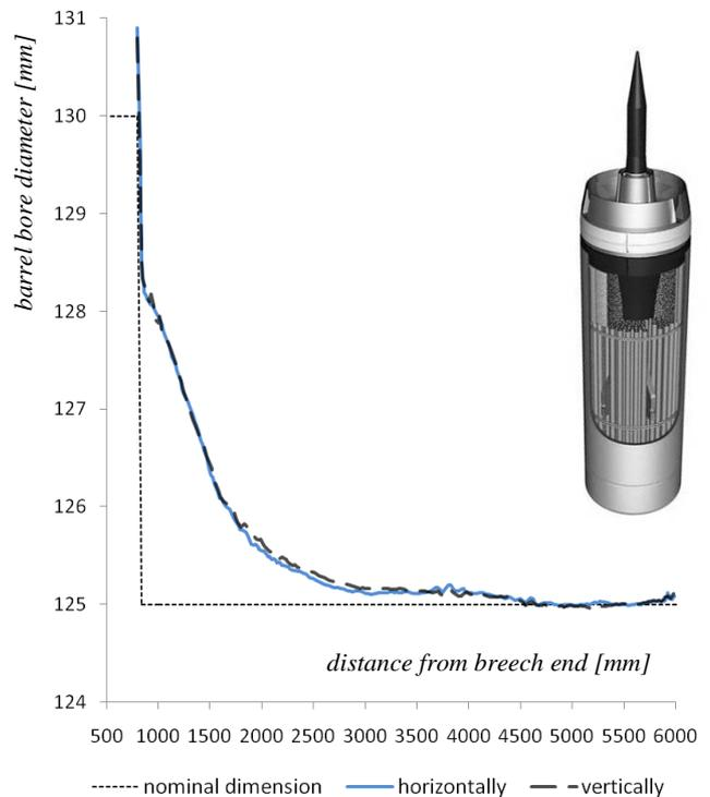
Fig. 4 Barrel No D0034 – wear caused predominantly by TAPNA projectile
