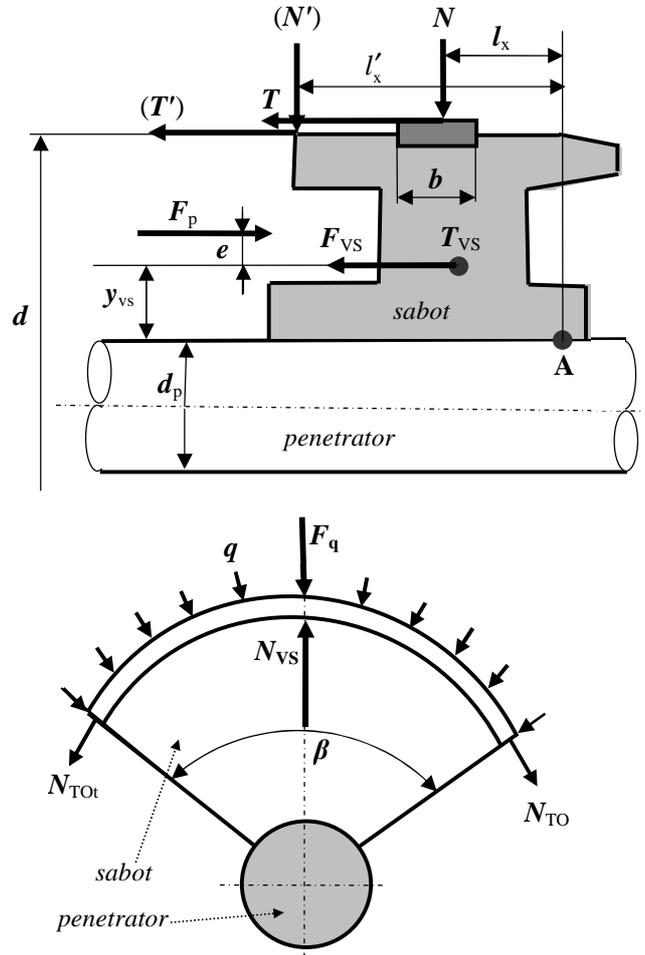
Fig. 5 Simplified diagram of forces affecting sabot of 3BM-9 and 3BM-15 projectiles
