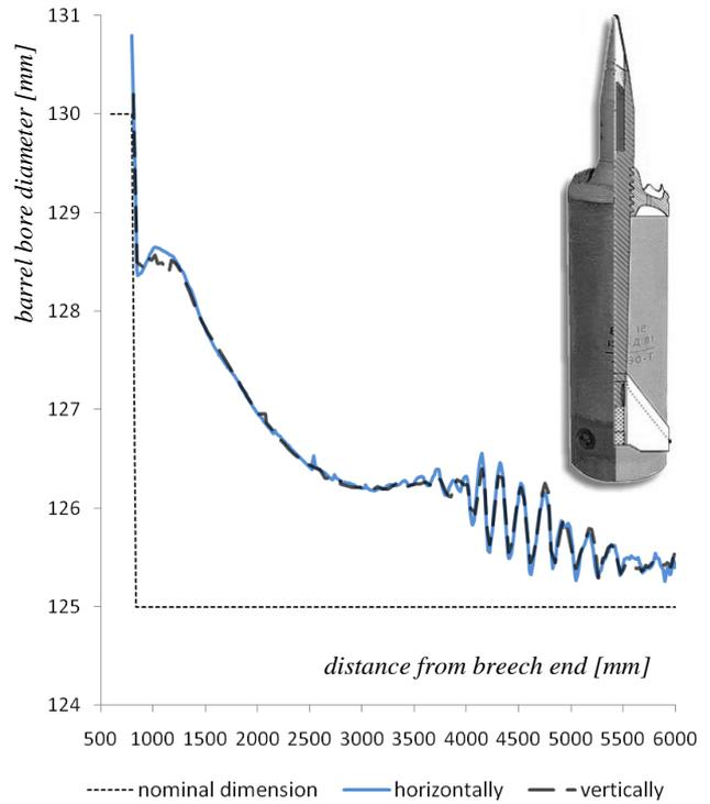
Fig. 3 Barrel No C0164 – wear caused by shooting mostly 3BM-15 and 3OF-19 projectiles
