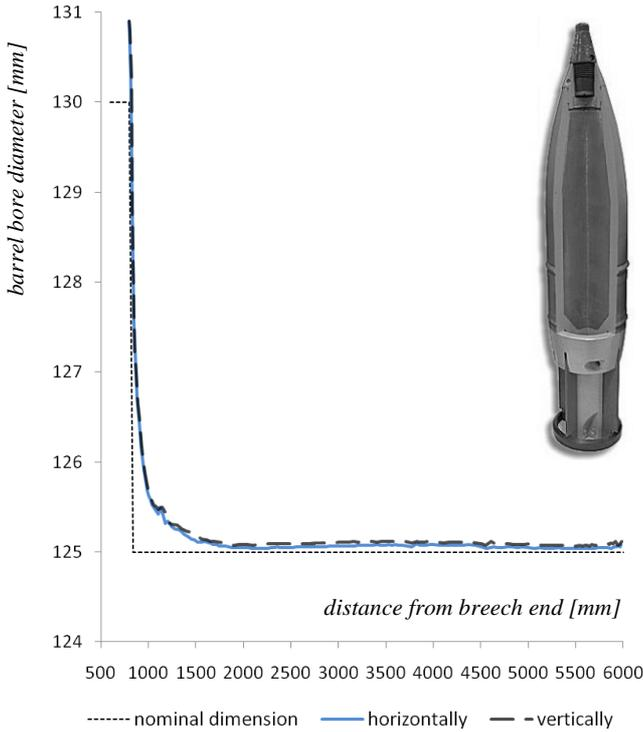
Fig. 2 Barrel No B0507 – wear caused mostly by 3OF-19 projectiles
