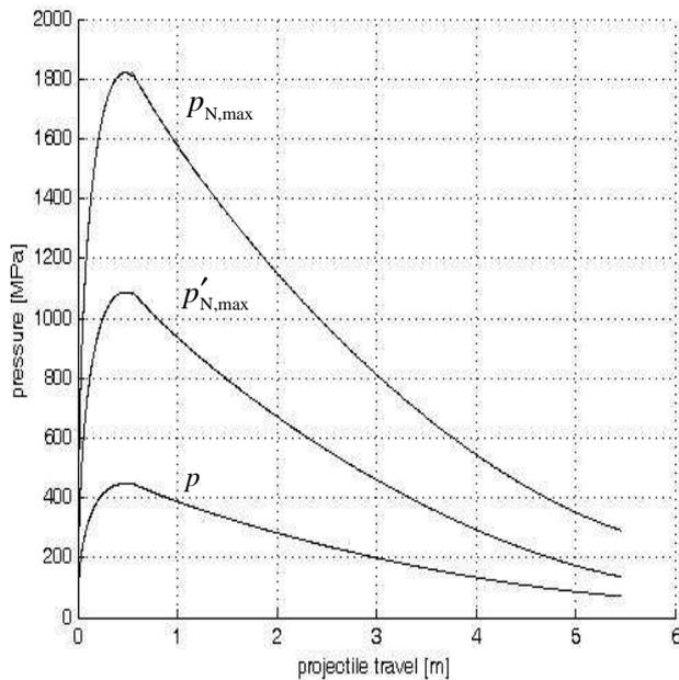
Fig. 6 Course of pressure of gases  $p$ , pressures  $p_{N,max}$  and  $p'_{N,max}$  in dependence on travel of seal ring in barrel
