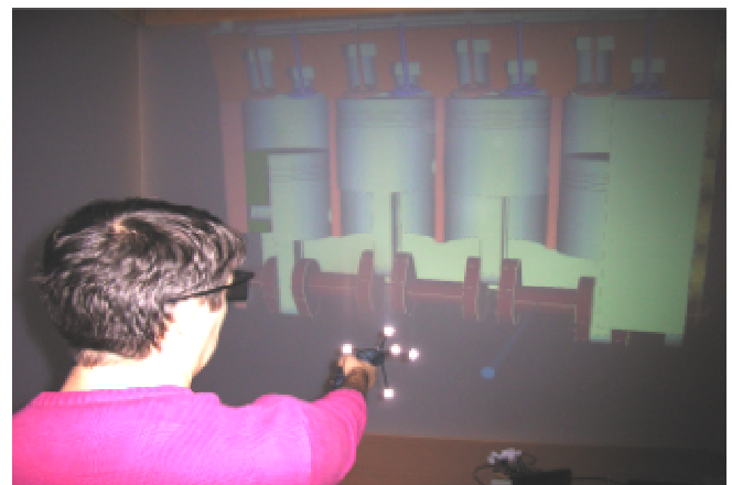
Fig.2 Inspection of a CAD model in immersive CVE
