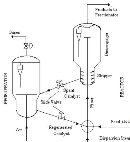
Fig. 1. The industrial fluid catalytic cracking unit.
