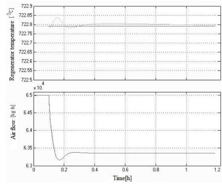
Fig. 10. The evolution in time of the regenerated catalysts temperature and air flow when the feedstock increases from the  $195^{\circ}C$  to  $215^{\circ}C$ .
