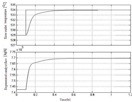
Fig. 7. The dynamic evolution of the riser outlet temperature and regenerated catalyst flow when the controller setpoint -  $T_r$  increases from  $529^{\circ}C$  to  $534^{\circ}C$ .
