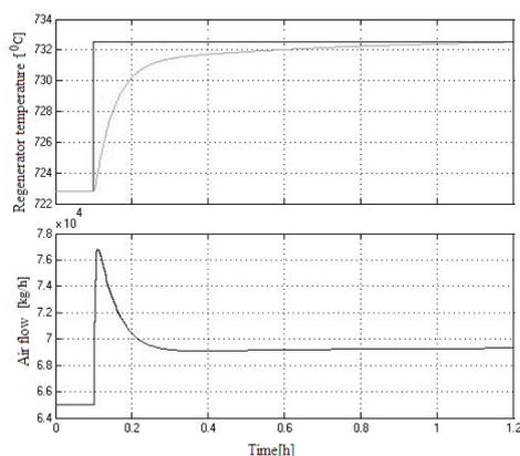
Fig.12. The dynamic evolution of the regenerator temperature and air flow trend when the temperature regenerator controller set point increases from 722.97 °C to 732.97 °C and the control interval is 0.0024h.
