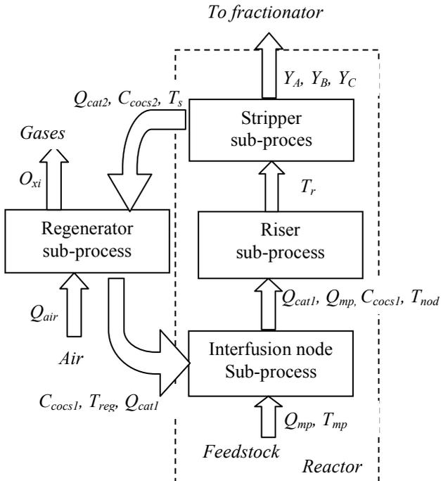
Fig. 2. The sub-process of the FCC.
