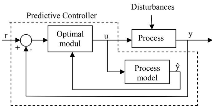
Fig. 5. The MBPC structure.
