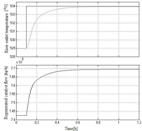
Fig. 11. The dynamic evolution of the riser outlet temperature and regenerated catalyst flow when the temperature riser controller set point increases from  $529^{\circ}C$  to  $534^{\circ}C$  and the control interval is  $0.024h$
