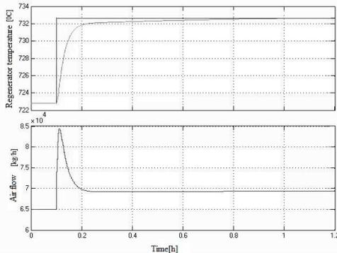
Fig. 8. The dynamic evolution of the regenerator temperature and air flow rate when controller set point -  $T_{reg1}$  increases from  $722.97^{\circ}C$  to  $732.97^{\circ}C$
