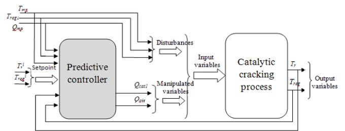
Fig. 6. The predictive control structure of the catalytic cracking process
