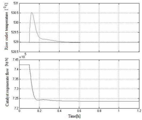
Fig. 9. The dynamic evolution of the riser outlet temperature and regenerated catalyst flow when the feed stock temperature increases from  $195^{\circ}C$  to  $215^{\circ}C$
