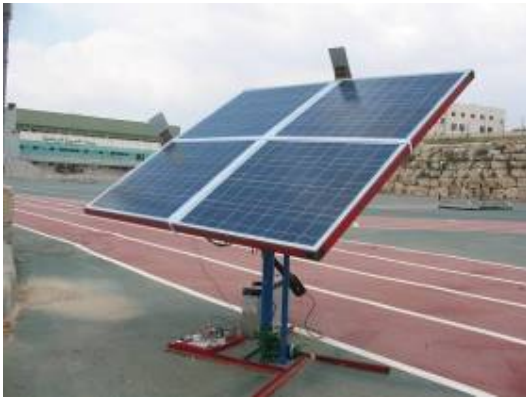
Fig.3. Birzeit Setup of solar tracker
