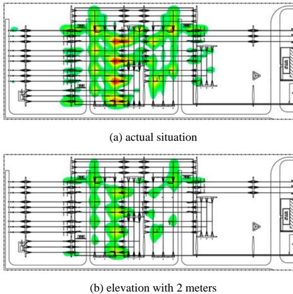
**Fig. 5.** Areas with field values higher than 10 kV/m
