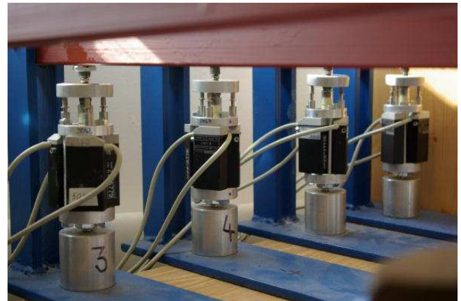
Fig.3: Lever mechanism – device for testing creep of homogenous materials.
