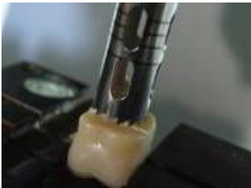
Fig.1 JMA Dakar device (clamping jaws, trepan bur, acrylic tooth).
