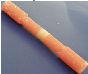
Fig. Nr.10. The shape and size of the sample corresponding to specification ADA / ANSI No.15
