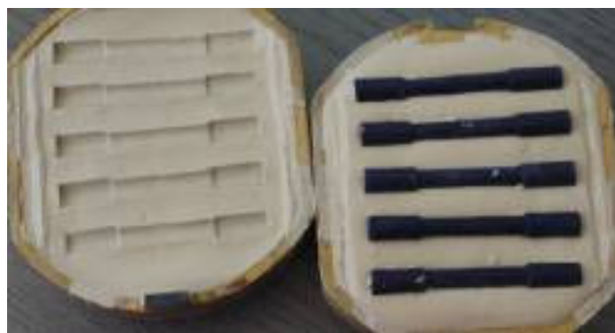
Fig. 7. Wax samples removed from plaster models.
