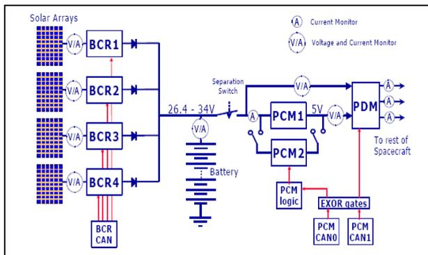
Fig 2 Alsat-1 power system block diagram.
