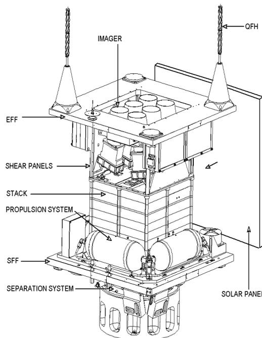
Fig 1 Alsat-1 platform architecture.
