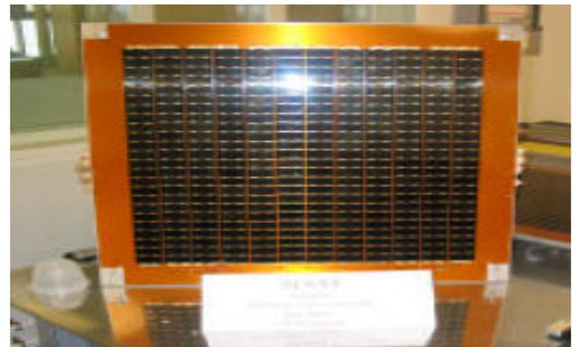
Fig 3 Alsat-1 flight model panel.
