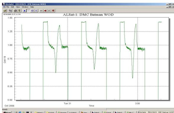
Fig 5-b Cell 19 acting as a resistor 30/10/2006.
