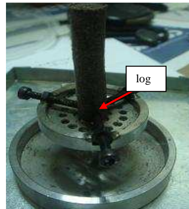
Fig. 1 Holder with Log or Briquette for Combustion Study
