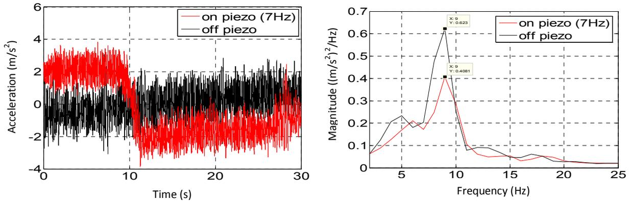
(a) Acceleration response when piezoelectric actuator vibrates at 7Hz
