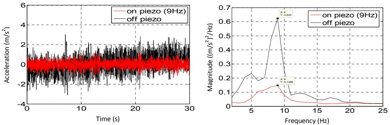
(c) Acceleration response when piezoelectric actuator vibrates at 9Hz
