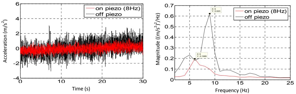
(b) Acceleration response when piezoelectric actuator vibrates at 8Hz
