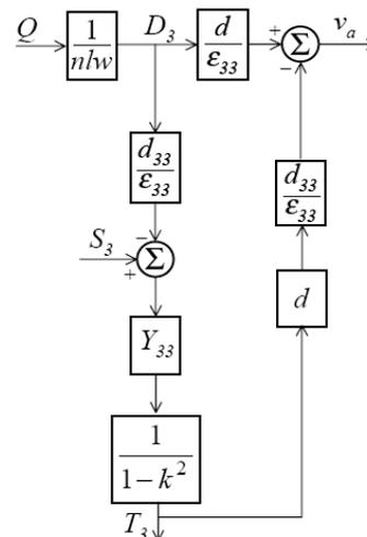
Fig. 2. Electromechanical model of piezoelectric actuator [16]
