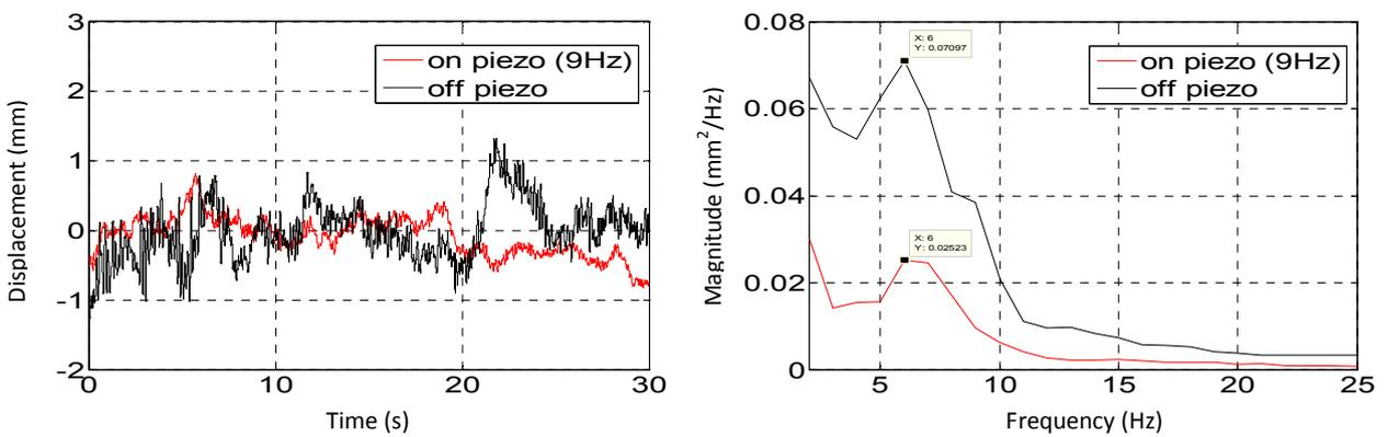
(c) Displacement response when piezoelectric actuator vibrates at 9Hz
