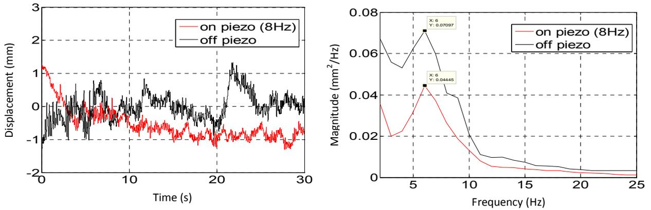
(b) Displacement response when piezoelectric actuator vibrates at 8Hz
