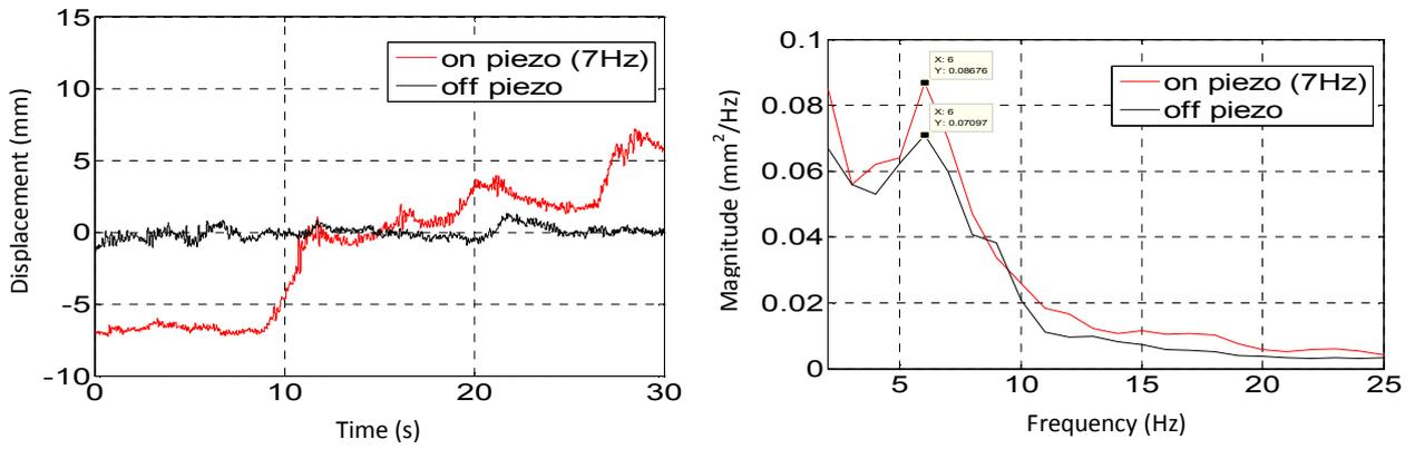
(a) Displacement response when piezoelectric actuator vibrates at 7Hz
