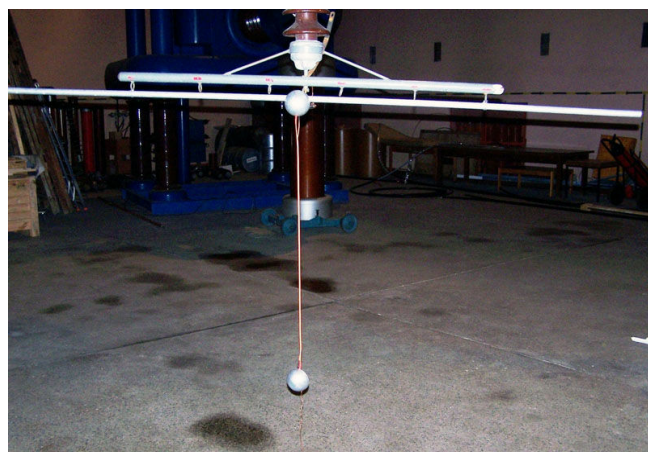
Fig.5 Withstand voltage tests
