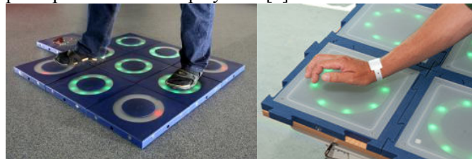
Fig. 1. Modular interactive tiles used for playful physiotherapy with feet or hands.
