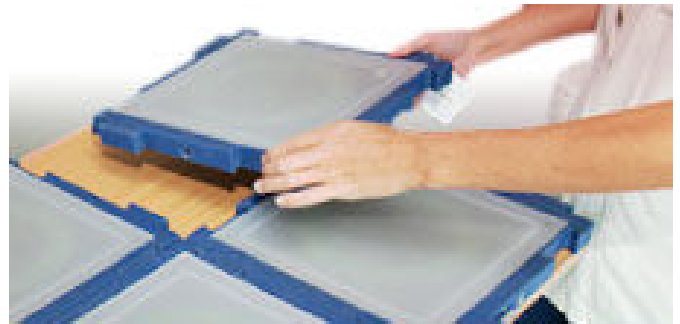
Fig. 3. Assembly of the modular interactive tiles as a simple jigsaw puzzle.
