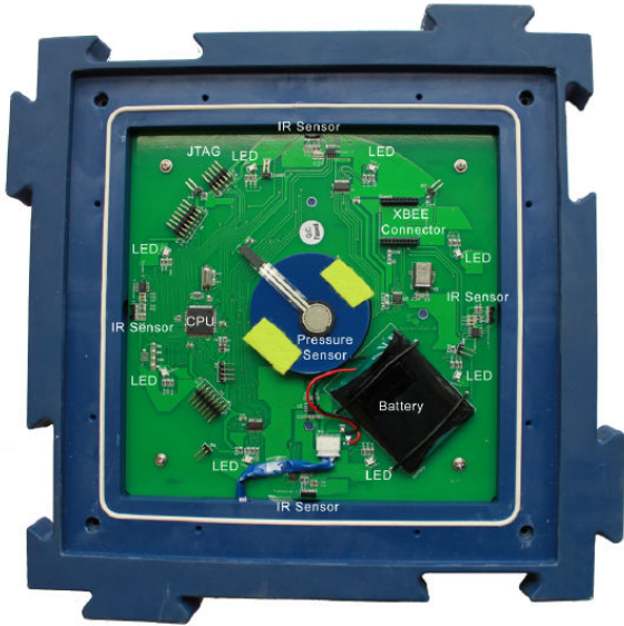
Fig. 2. PCB and components of a modular interactive tile.
