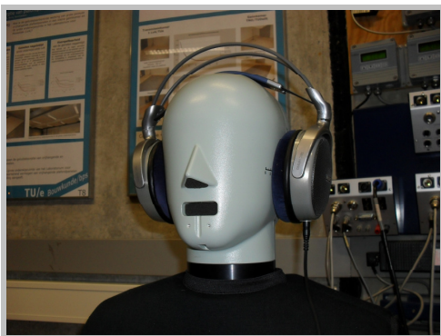
Fig 5. Headphone transfer measurement using a HATS.
