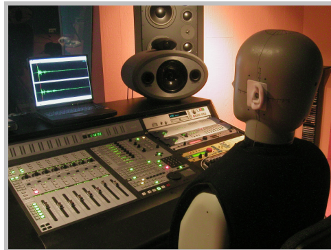
Fig 4. Sweet spot measurement using a Head and Torso Simulator (HATS) or an artificial head.
