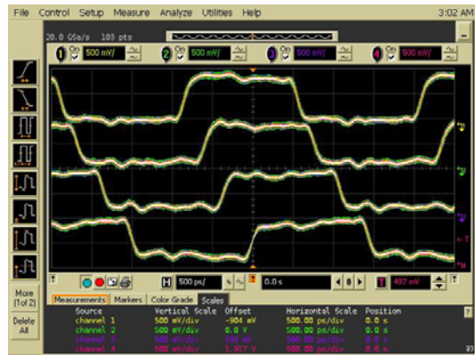
Fig. 7. Multi-phase clocks of PLL
