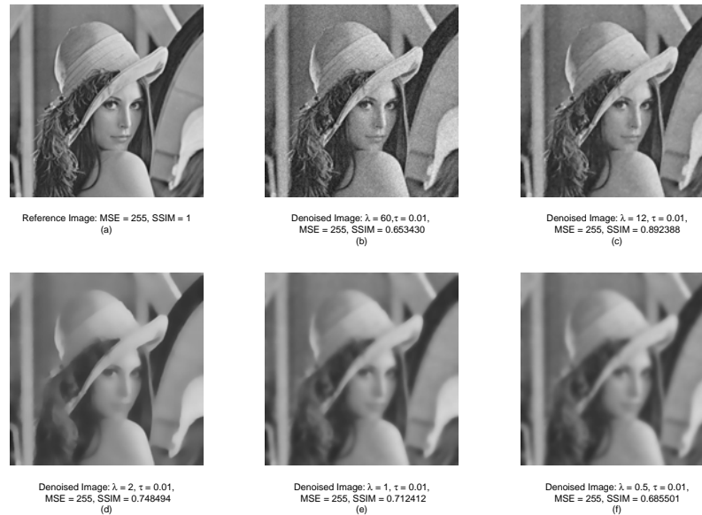
Figure 2: Denoised images showing values MSE values and SSIM index values
