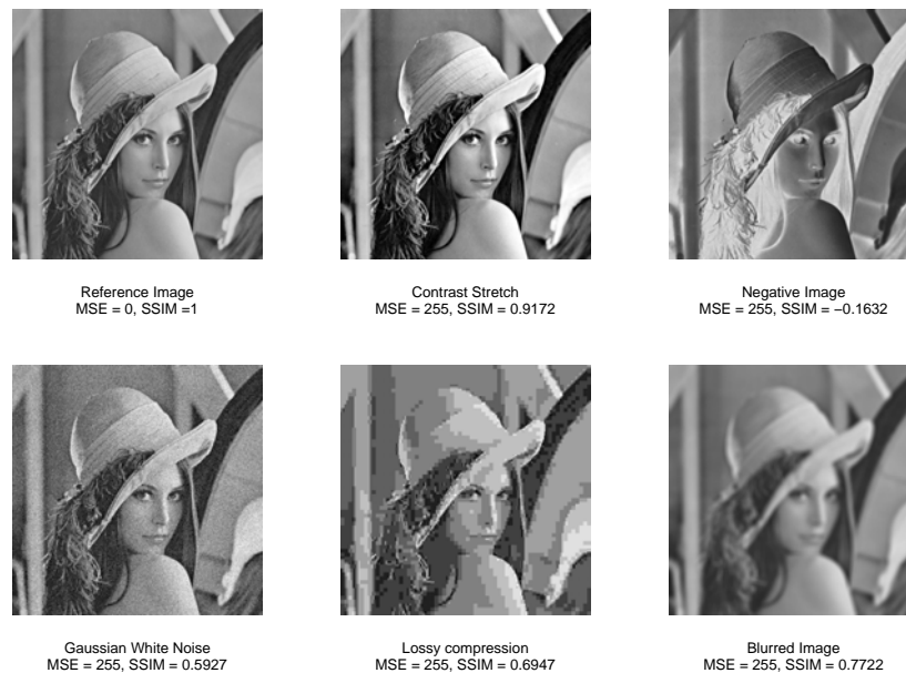
Figure 1: Images with different structural distortions but the same MSE values
