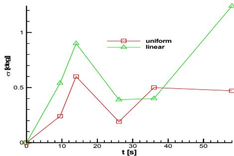
Fig. 14 Climb angle diagram, standard deviation values, low turbulence
