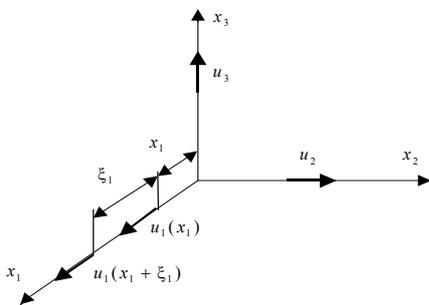
Fig. 1 Longitudinal correlation of velocity components
