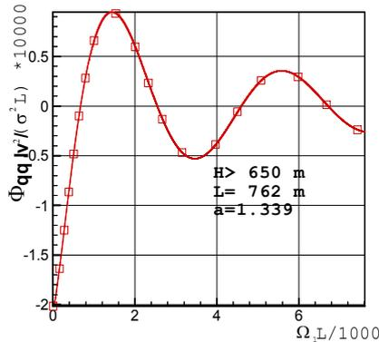
Fig. 8 Spectral function for the rotation velocity
