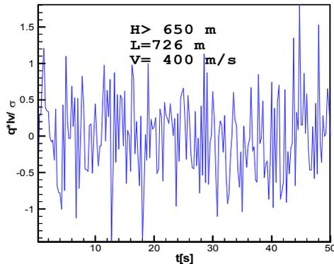
Fig. 10 The pitch velocity produced by turbulence
