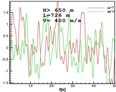
Fig. 9 The axial  $u_g$  and normal  $w_g$  velocities produced by turbulence
