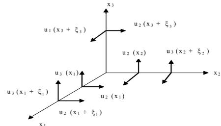
Fig. 2 Transversal correlation of velocity components
