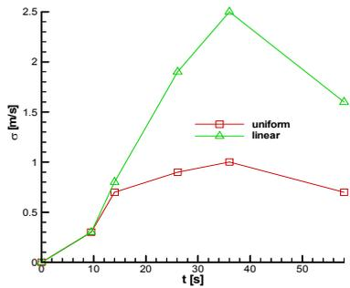
Fig. 12 Velocity diagram standard deviation values, low turbulence
