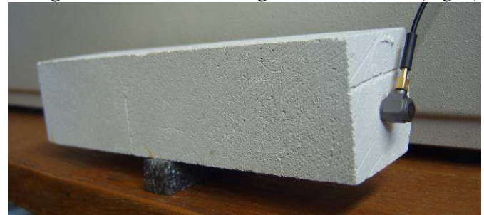
Fig. 2 The test arrangement for measuring the fundamental longitudinal resonant frequency of the gypsum specimen
