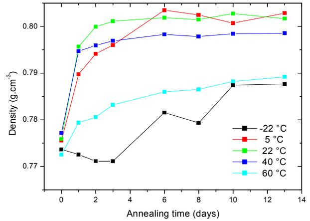
**Fig. 1** Evolution of density in compression-molded specimens with thickness of 0.5 mm, 1 mm, 2 mm (down from top) of PB0300M
