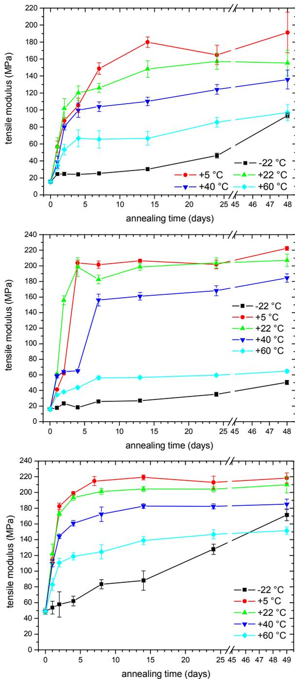
**Fig. 4** Evolution of tensile modulus in injection-molded specimens of PB 0300M, DP 0401M and PB 8640M (down from top)
