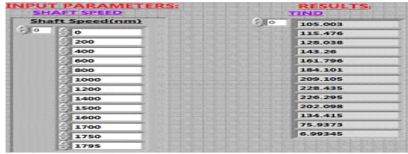
Fig. 22. Input parameters and Results for torque speed relationship of an induction motor
