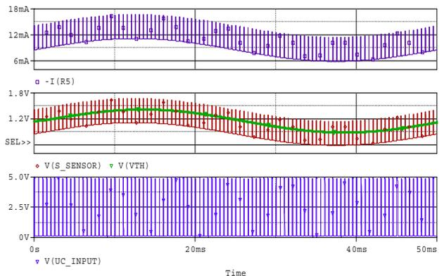
Fig.10. Proposed circuit threshold adapting behavior simulation
