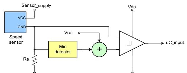
Fig. 7. Proposed circuit block diagram
