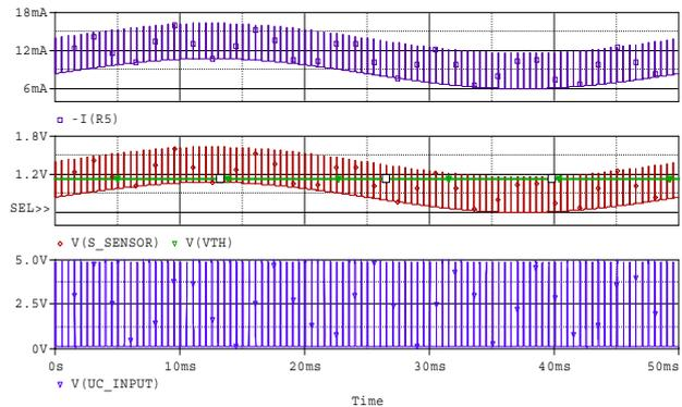
Fig. 6. Typical circuit behavior at sensor supply current limit ranges of a typical speed sensor.
