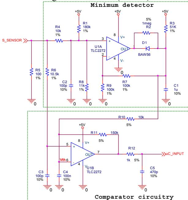
Fig. 8. Proposed interface circuit schematic
