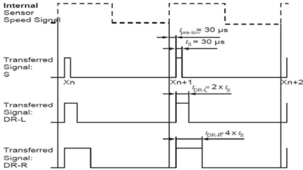
Fig. 3. Output signal and direction encoding
