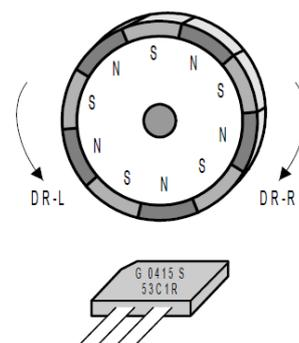
Fig. 2. Infineon speed sensor concept
