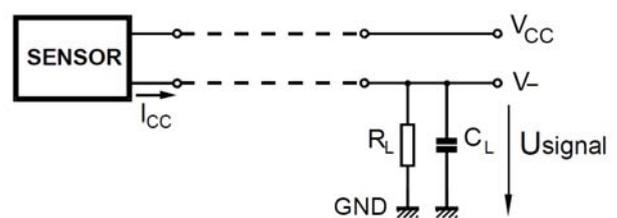
Fig. 1. Two wire speed sensor interconnecting diagram
