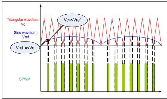
Fig. 2 Cross over point to generate SPWM
