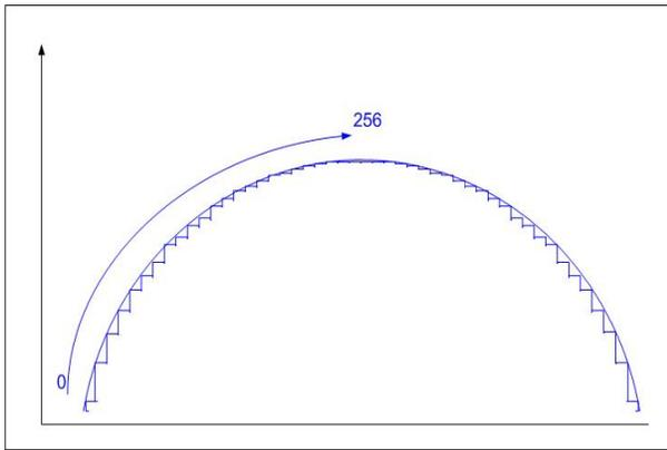
Fig. 8 Sine wave with 256 quarter for number of bit 8
