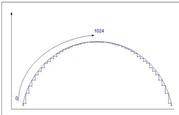
Fig. 9 Sine wave with 1024 quarter for number of bit 10
