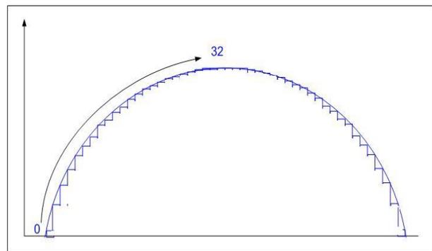
Fig.7 Sine wave with 32 quarter for number of bit 5
