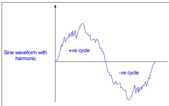
Fig. 4 Sine waveform with harmonic
