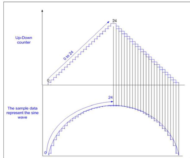
Fig. 6 Sine waves produce by quarter cycle
