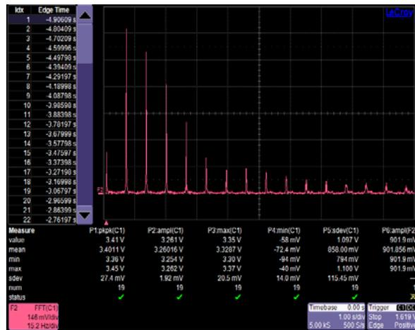
Fig. 10 Converting SPWM to Fast Fourier Transform (FFT) wave.
