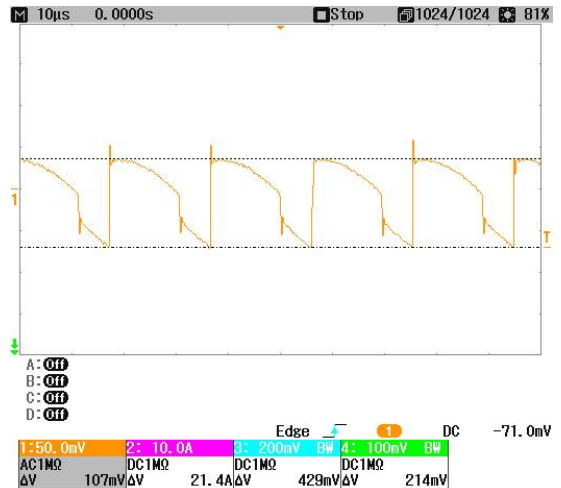
Fig. 5. Output voltage ripple with 100µF Al-SC.
