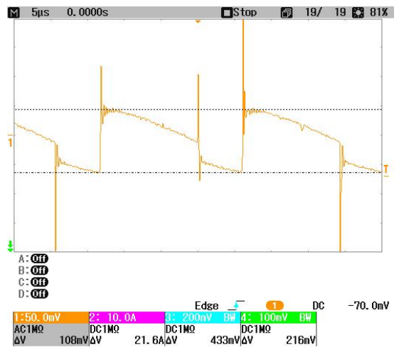
Fig. 6. Output voltage ripple with 220µF (S.H.I.).
