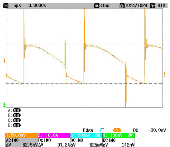
Fig.7. Output voltage ripple with 470µF series Ta.
